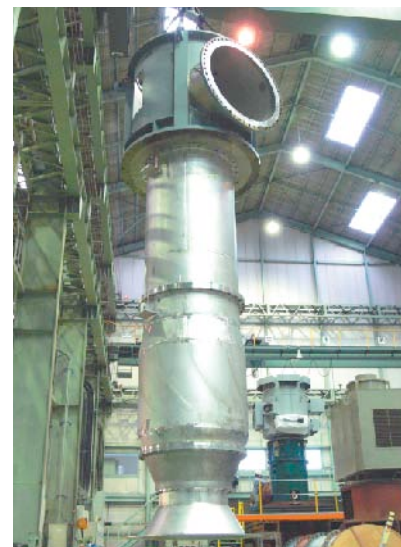
Circulating water pump for Mesaieed A IWPP project, Qatar (Size:1,500mm, Driver:1,650kW)
