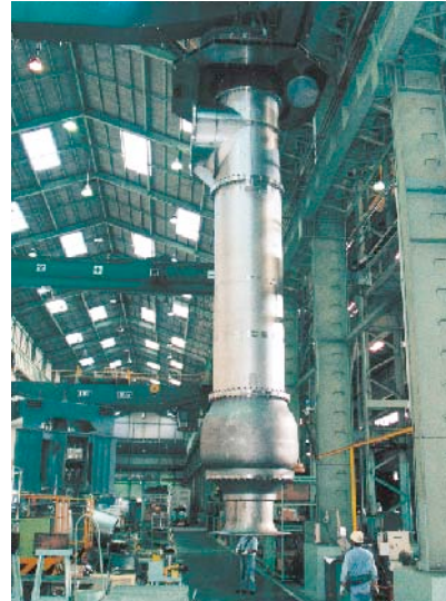
Cooling water pump for P.A.I. Shuaiba, Kuwait (Size:1,400mm, Driver:1,500kW)
