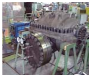
Hydraulic pressure test
