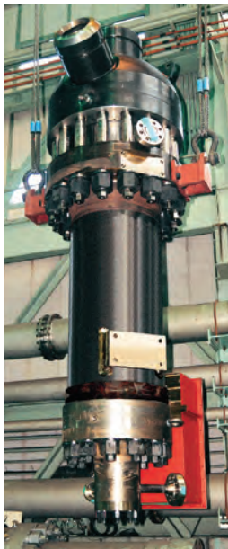
φ 250 Boiler circulation pump (KEPCO, PUSAN COMBINED CYCLE POWER PLANT, KOREA)
