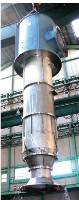
φ 1400 FGD Absorber pump (JIMAH POWER PLANT, MALAYSIA)
