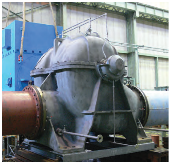
φ 1000 Circulating water pump (BLUEWATERS POWER STATION UNIT 1 PROJECT, AUSTRALIA)
