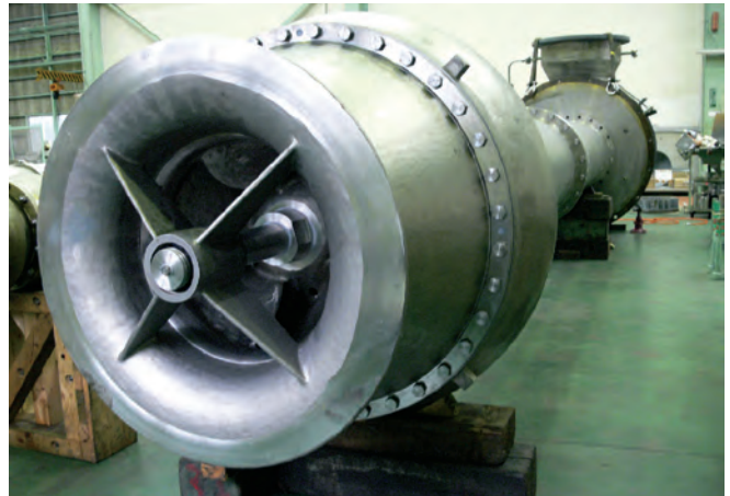
φ 900 Seawater pump (SOUSSA DESALINATION PLANT, LIBYA)
