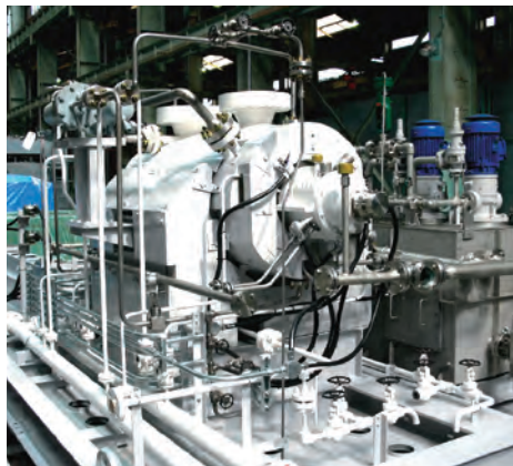
HP Barrel type feed pump acc. to API 610 (SAUDI KAYAN PETROCHEMICAL COMPANY, SAUDI ARABIA)
