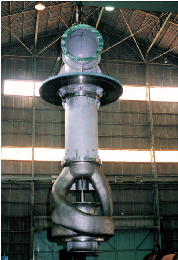
φ 900 Hot well pump (OLAKARIA II GEOTHERMAL POWER PLANT, KENYA)
