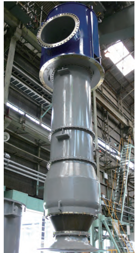
φ 1350 Circulating water pump (SAN MARTIN CCPP, ARGENTINE)
