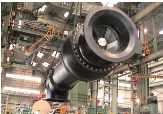
φ 1500 Seawater supply pump (SABIA DESALINATION PLANT III, KUWAIT)
