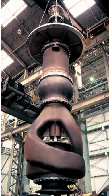
φ 1100 Brine recirculation pump (AL SHOAIIBA PHASE 2, SAUDI ARABIA)
