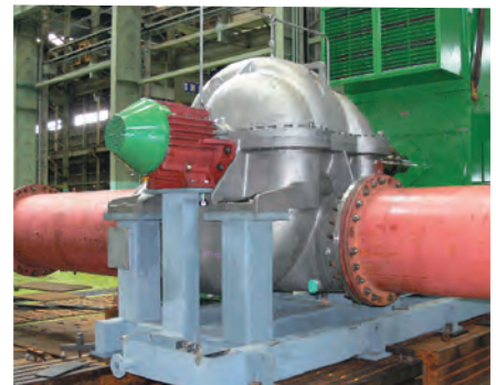
φ 900 x 700 UF feed pump (SHUWAIKH RO PJT, KUWAIT)
