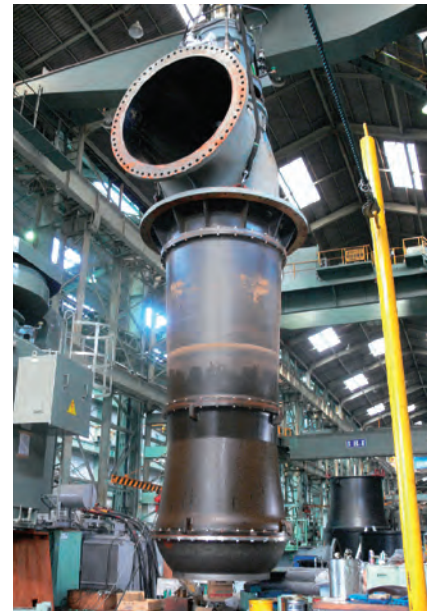
φ 1500 Main circulation water pump with adjustable vane (OMON THERMAL POWER PLANT, VIETNAM)
