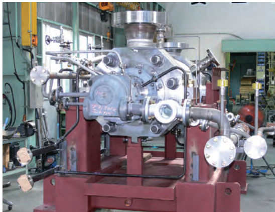
Boiler feed water pump (XIAMEN CCGT POWER PLANT 350MW CCGP x 2, CHINA)
