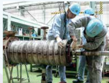
Overhaul of a multi-stage ring section pump
